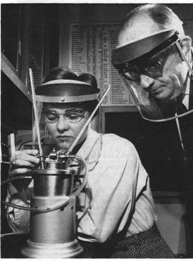
FLASH POINT of highly volatile liquids is determined by Mina Carnicom (3211) through use of a tag closed cup tester as Safety Engineer J. E. Baylor (3210) looks on. Thermometers indicate heat rise of sample and water bath in cylinder. Proprietary products containing acetone or various alcohols are among liquids tested in container such as this.
